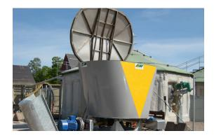
System suitable for the processing of various biodegradable materials, such as: manure, vegetable processing scraps, agricultural by-products, silage. The material is mixed and shredded by blades bolted to the mixing screw. Discharge can be applied on the bottom of the tank, side wall or front. Manually or hydraulically activated discharge door (where applicable).
